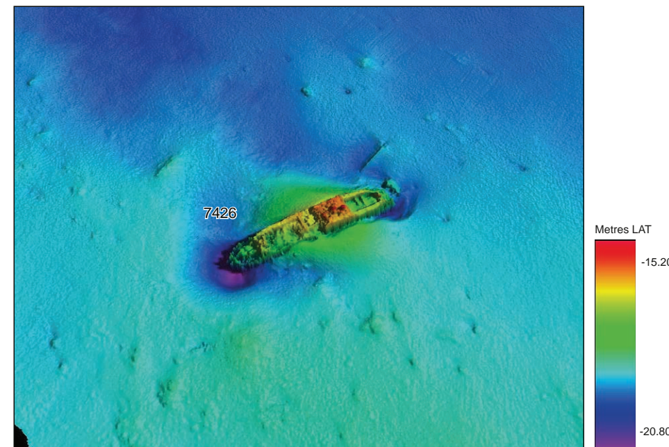
MBES grid image, x 1 vertical exaggeration, looking south-west
